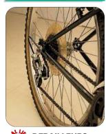
Marailleurs (named from the French word meaning 'derail') move the chain among two to six sprockets of different diameters to change gears.
