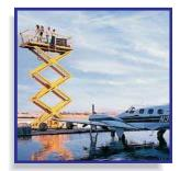
🦠 SCISSORS LIFT Photographers can use scissors lifts for overhead shots, as shown at the left. The crossing beams of the lift form parallelograms that move together to raise and lower the platform. In Exercises 51-54, use the diagram of parallelogram ABDC at the right.
